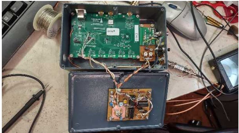
The Beacon Blaster and the BPSK modulator/PIC IDer in the lid. This photo was taken prior to the addition of the "T2" carrier circuitry. The combiner and MMIC amplifier may be seen on the far right of the chassis.
