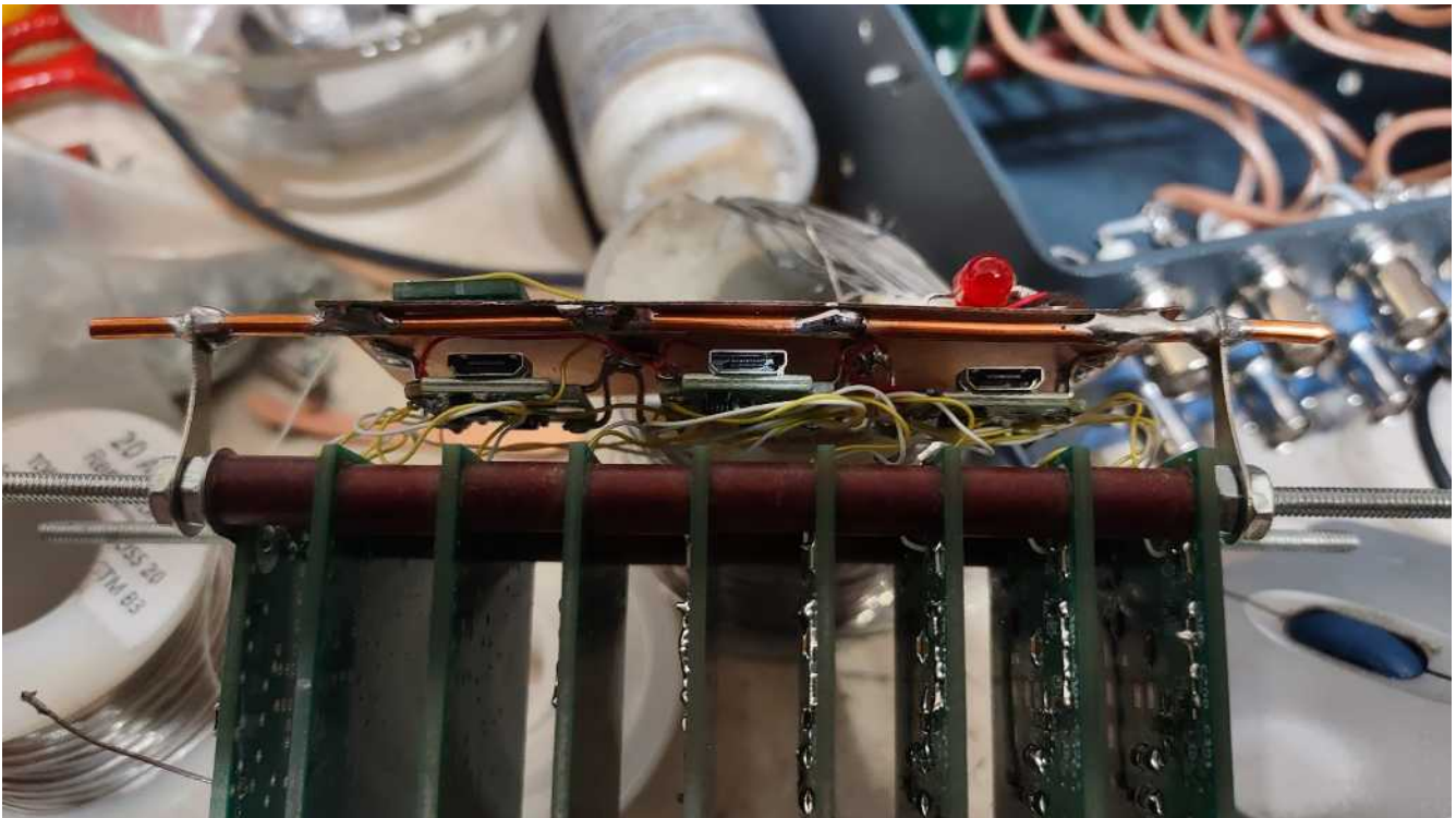
The three Progrock 2 Si5351 modules mounted to the stack of converter boards. Just barely visible is the clock multiplier board, seen edge-on on the top side of the board. The "clock switch" board - to the right of the multiplier - is not visible.
