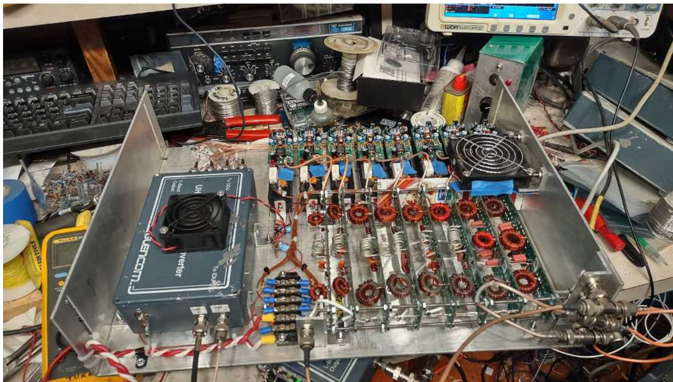
The complete multi-band chassis - sans the 45 MHz exciter. In the background are the eight QRP-Labs 10 watt amplifiers: A ninth amplifier was built and tested as a ready spare.
