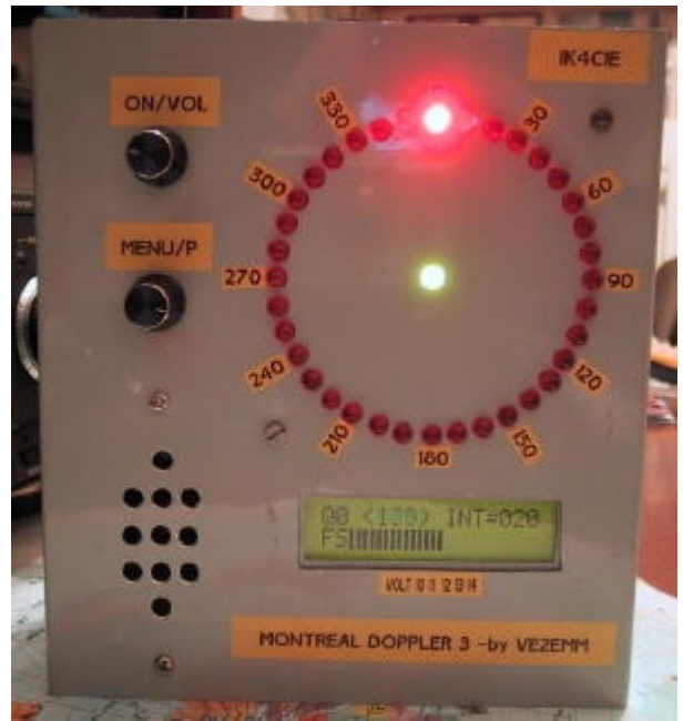
THE "FS" BARGRAPH USED AS A BATTERY MONITOR
